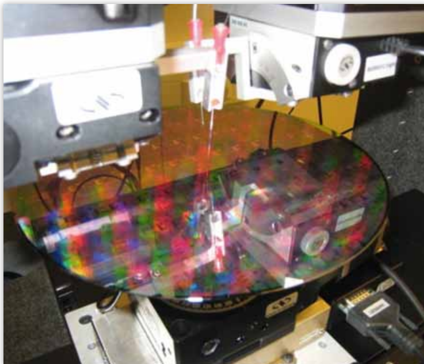
Wafer-scale test of silicon photonic IC © Ghent University–imec
