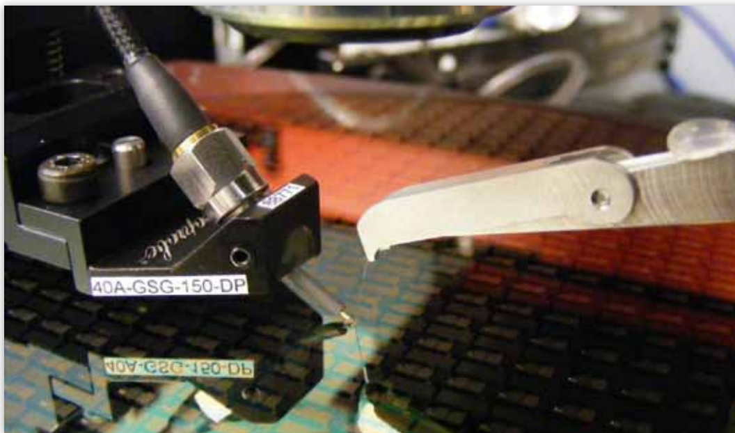
High frequency wafer level testing of germanium photodiodes on silicon. © CEA-Leti
